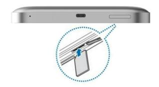
Insert the SIM card into the slot.
